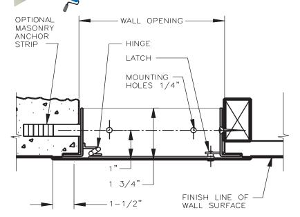
This precision-flush access door for wall and ceiling installation far surpasses other doors. Laser cut from one sheet of cold rolled steel, no corner mitering - aesthetically preferred by architects and building professionals.
